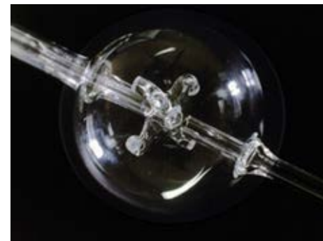
Jet stirred reactor for gas-phase reactions
