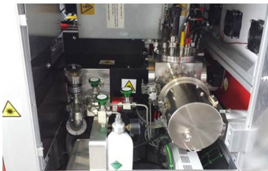
Photoionisation mass spectrometry for on-line analysis of tar
