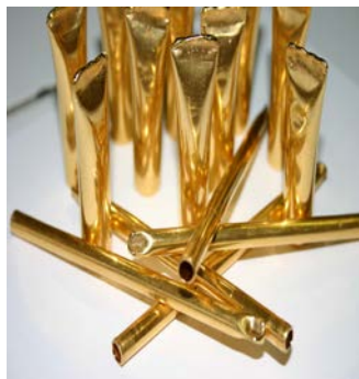
Gold cells for high pressure pyrolysis
