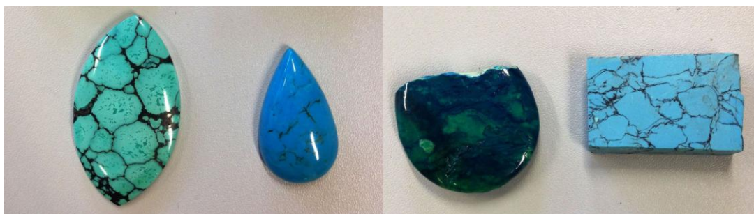
Fig. 1. Different turquoise samples, from left to right : chinese matrix turquoise, polymer stabilized turquoise, polyurethane coated stone, turquoise stabilized with melamine resin.
